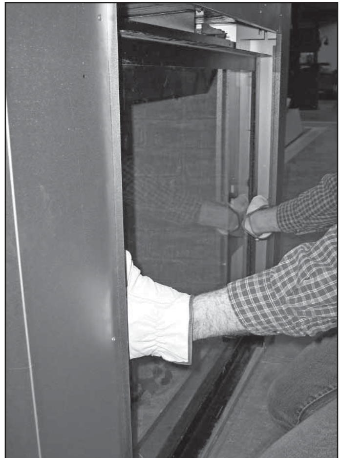
Figure 15.9 Lift Glass Frame Assembly Forward
